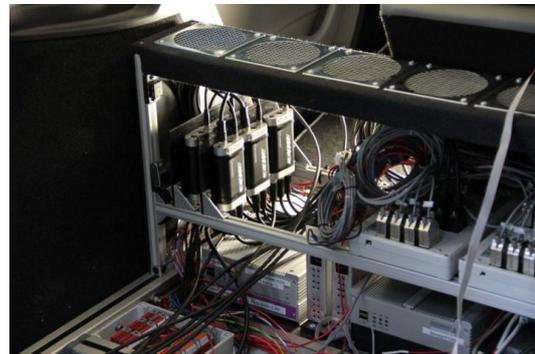
CatchTheBus as FlexRay-to-CAN gateways for a Steer-by-Wire application in a highly automated vehicle
